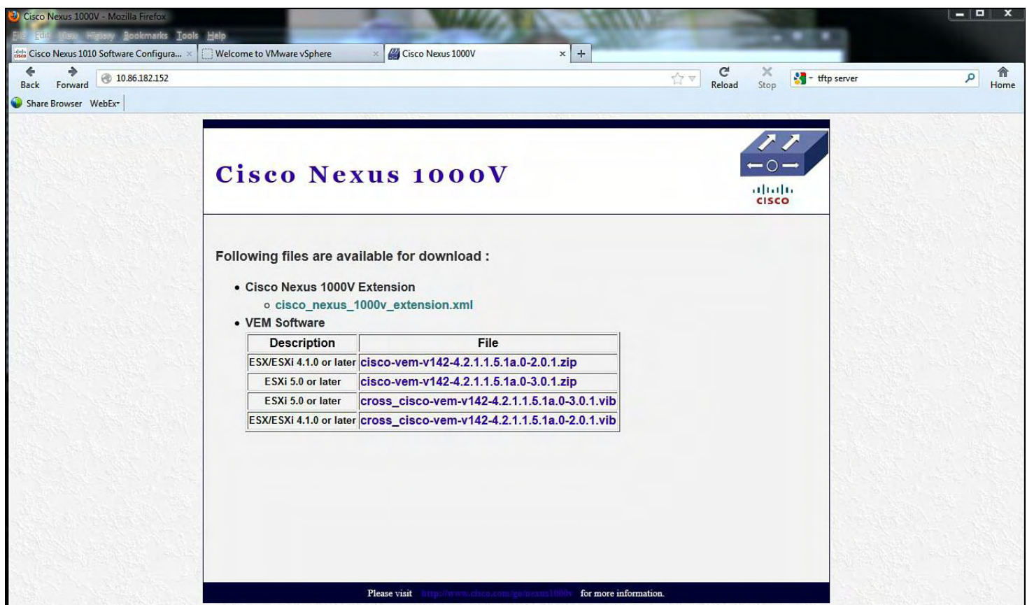
Figure 9-4. Launching the Web Browser on the vCenter Server and Pointing to the mgmt0 Interface of the VSM
