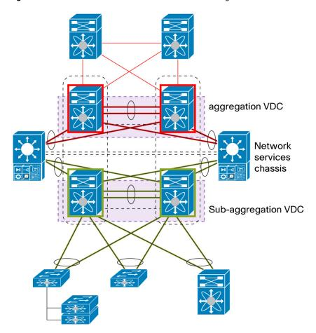
Figure 70. Network Services Chassis with VDC Sandwich Design
