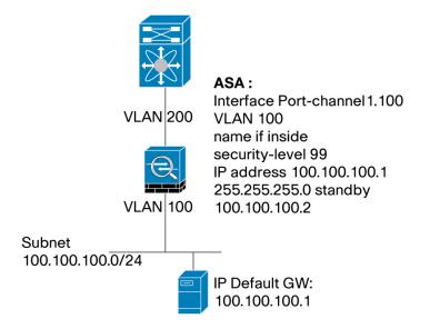
Below is a sample port-channel configuration for ASA in routed mode:
