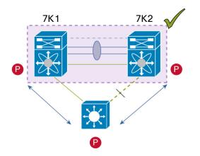
Figure 54. Supported Designs for Layer 3 and vPC: Peering over a Spanning Tree Protocol Interconnection Using a non-vPC VLAN
