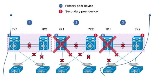
Figure 95. vPC Auto-Recovery - vPC Peer-Link Failure Then vPC Primary Peer Device Failure
