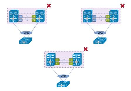
Figure 19. Unsupported Configurations for vPC Peer-Links (Both Sides Must Be of Same Port Type)
