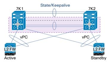
Service appliance in transparent mode behaves like a bump in the wire and bridge traffic from inside interface to outside interface by swapping the VLAN id. Note that ingress VLAN and egress VLAN are associated to the same IP subnet.
