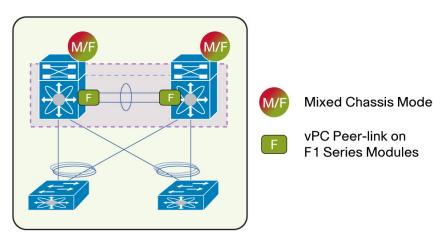
Figure 91. vPC Peer-Gateway Exclude-VLAN - Unique Topology Where the Feature Apply
