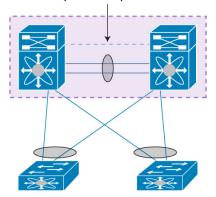
The vPC peer-keepalive link carries periodic heartbeat between vPC peer devices. It is used at the boot up of the vPC systems to guarantee both peer devices are up before forming vPC domain and also when vPC peer-link fails to down state; in the latter case, vPC peer-keepalive link is leveraged to detect split brain scenario (both vPC peer devices are active-active) [when vPC peer-link is down, there is no more real time synchronization between the 2
