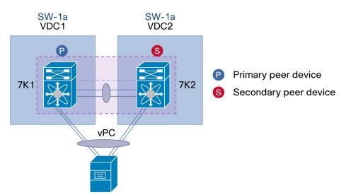
Figure 86. vPC Domain Created Within the Same NEXUS 7000 Chassis Using 2 Different VDC
