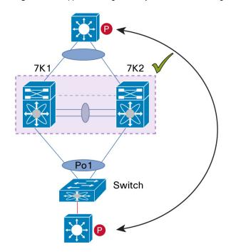
In this design, vPC is used as a pure L2 transit path. Because there is no direct routing protocol peering adjacency from L3 device to any vPC peer device, this topology is entirely valid and fully supported.
