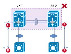
L3 device single-attached to vPC domain using vPC VLAN is not a supported design.
