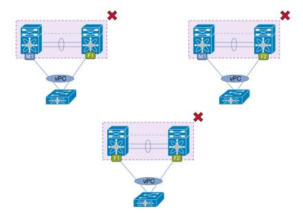
**Note:** M132XP and M108X2 (32 10-Gigabit Ethernet line cards and 8 10-Gigabit Ethernet line cards, respectively) can form a port-channel together and then can co-exist in the same vPC member port. However, be aware of the requirement that ports on M132XP can form a port-channel or vPC member port with ports on M108X2 only if M132XP ports are configured in dedicated mode.
