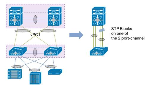
Figure 33. Incorrect Configuration of Double-Sided vPC Topology
