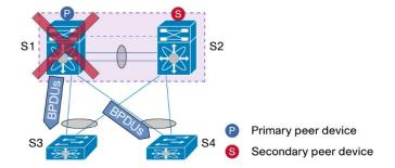
Figure 47. Using Bridge Assurance (BA) on vPC
