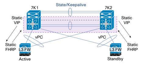
In this design (figure 75), L3 service appliance is vPC-attached to each vPC peer device.
