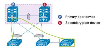
If you can't use an intermediate vPC-attached switch or VDC, the next best alternative is to connect the device to vPC peer devices using a non-vPC VLAN (by definition, a non-vPC VLAN is a VLAN that is not part of any vPC and then not present on vPC peer-link) and create a dedicated inter-switch port-channel to carry these non-vPC VLAN (figure 35).
