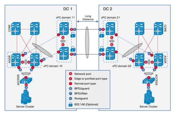
Figure 37. Multilayer vPC for Aggregation and DCI
