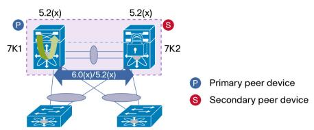
In Step 1, as Figure 88 shows, both vPC peer devices run the Release 5.2 code. Release 6.0 code is loaded on vPC peer device 1, 7K1 (loading the code first on primary or secondary vPC peer device has no importance) using ISSU. Note that other vPC peer device (7K2) has its configuration locked to protect against any operation on the switch.
