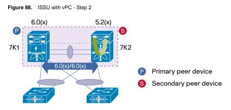
In Step 2, vPC peer device 1 (7K1) is now loaded with NX-OS Release 6.0. vPC peer device 2 (7K2) now loads the Release 6.0 code using ISSU. 7K1 configuration is then locked to prevent any change during the upgrade.
