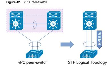
Most common mistake with vPC peer-switch deals with spanning tree configuration.
