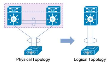
vPC leverages both hardware and software redundancy aspects:
