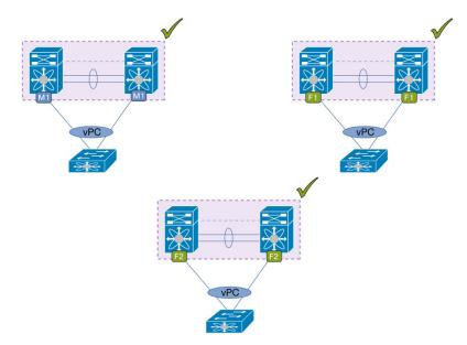
Figure 23. Supported Configurations for vPC Member Ports
