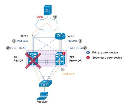
Figure 81. Multicast with vPC - PIM Prebuild SPT
