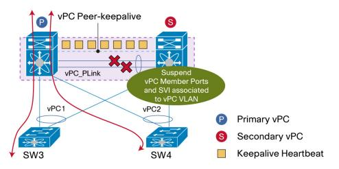
If orphan ports are connected to vPC secondary peer device, they become isolated once peer-link is down. In a VXLAN + vPC implementation, when a vPC peer-link shuts down, all Layer 2 or Layer 3 orphan receivers behind the non-forwarder (shut down vPC peer-link) will not receive any traffic.
