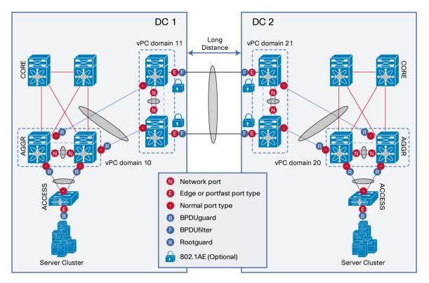
Another design is to interconnect directly between vPC aggregation layer, without using any dedicated vPC layer for DCI. This design is referred to as dual Layer 2 /Layer 3 pod interconnect and is shown in Figure 8.
