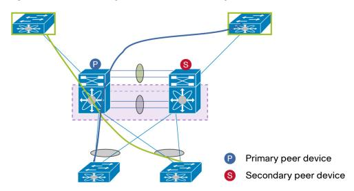
Figure 35. Access Device Single-Attached to vPC Domain Using Non-vPC VLAN
