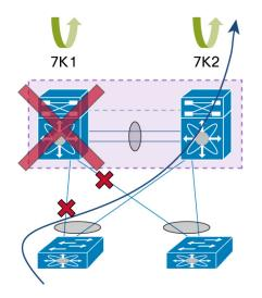
Figure 96. vPC Auto-Recovery Reload-Delay - Both vPC Peer Devices Reload But Only 7K2 Comes Back to Life
