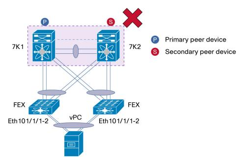
eVPC (enhanced vPC) is the configuration where FEX is vPC-attached to 2 different parent switches and server is vPC-attached to the 2 FEX (this design is also called 2-layer vPC). This is not supported on FEX with NEXUS 7000 series switches in vPC mode.
