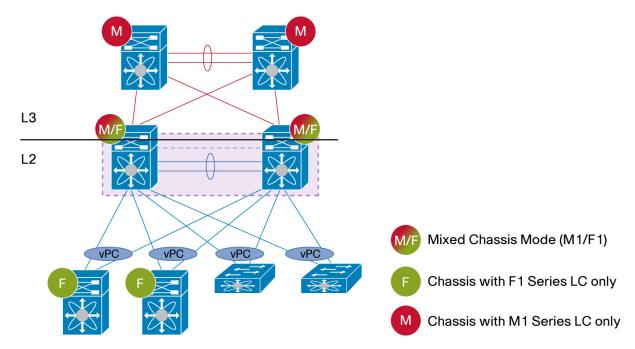
Figure 25. vPC System in Mixed Chassis Mode Configuration
