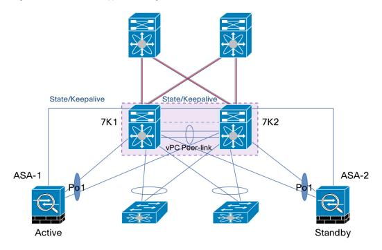
ASA-1 and ASA-2 run in HA (High Availability): ASA-1 is operating in active mode while ASA-2 is in standby mode. ASA-1 will process all flows coming from the network. If ASA-1 is down, ASA-2 will become active and then will be able to process subsequent flows.
