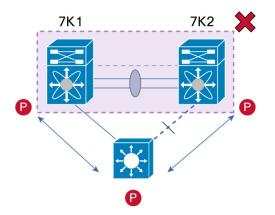
Connecting a L3 device to vPC domain using STP links with vPC VLAN is not a supported design.
