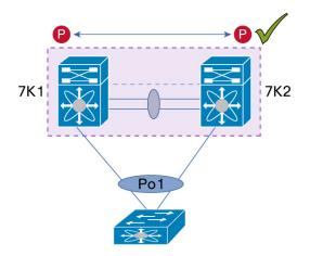
Peering between the 2 vPC peer devices is fully functional and primary use case for this type of design deals with L3 backup routed path. In case L3 uplinks on vPC peer device 1 or peer device 2 fail down, the path between the 2 peer devices is used to redirect traffic to the switch having L3 uplinks in UP state.
