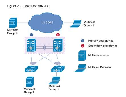
vPC uses Cisco Fabric Services (CFS) to synchronize Internet Group Management Protocol (IGMP) states. IGMP packets are sent with information about the source interface so that the equivalent state can be established on vPC members on both the vPC peers.
