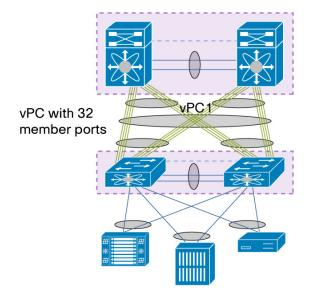
Figure 31. Double-Sided vPC with 32-Way Port-Channel
