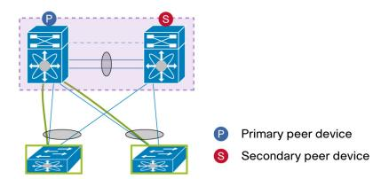
Figure 29. Access Devices Dual-Attached to a vPC Domain
