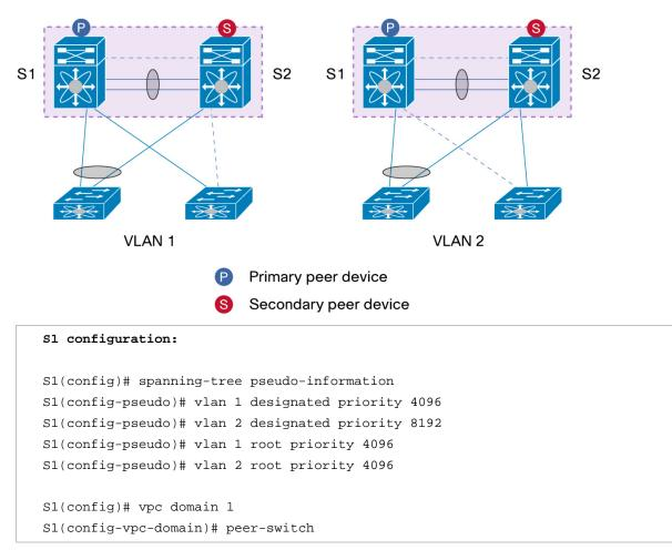
Figure 46. Hybrid Topology Reference for Peer-Switch with Spanning-Tree Pseudo-Information Configuration Sample
