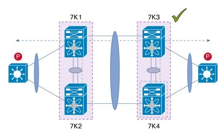
Figure 55. Layer 3 and vPC Supported Designs: Peering between Two Routers with vPC Devices as Transit Switches
