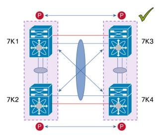
Figure 57. Layer 3 and vPC Supported Designs: Peering over a vPC Interconnection (DCI case) on Parallel Interconnected Routed Ports
