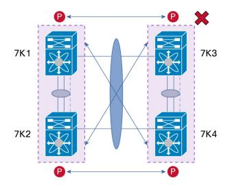
Figure 62. Layer 3 and vPC Unsupported Designs: Peering Over a vPC Interconnection (DCI Case)
