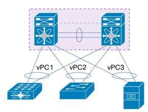
The access device can be any endpoint equipement (L2 switch, rack-mount server, blade server, firewall, load balancer, network attached storage [NAS] device). Only prerequisite for the access device is to support port-channeling (or link aggregation) technology:
