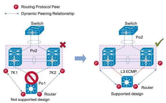
Figure 49. Using Separate Layer 3 Links to Connect L3 Device to a vPC Domain
