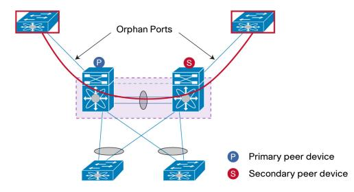
Figure 36. Access Device Single-Attached to vPC Domain Using vPC VLAN
