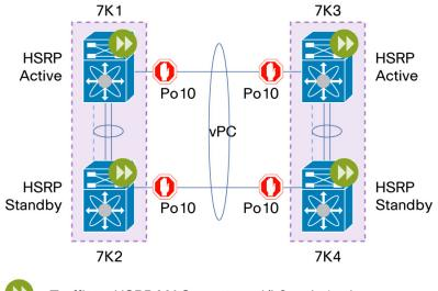
Figure 69. DCI with a Single HSRP/VRRP Group - Active/Active in DC1 and Active/Active in DC2
