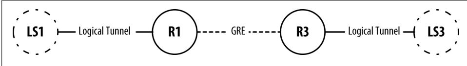
Figure 7-14. Tunnel Services Case Study: Logical End-to-End Connectivity.
