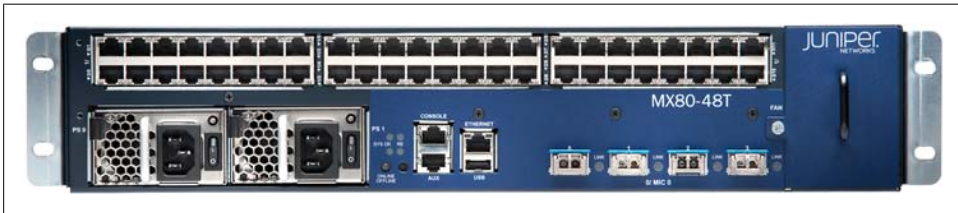
Figure 1-7. Juniper MX80-48T supports 48x1000BASE-T and 4x10GE ports
