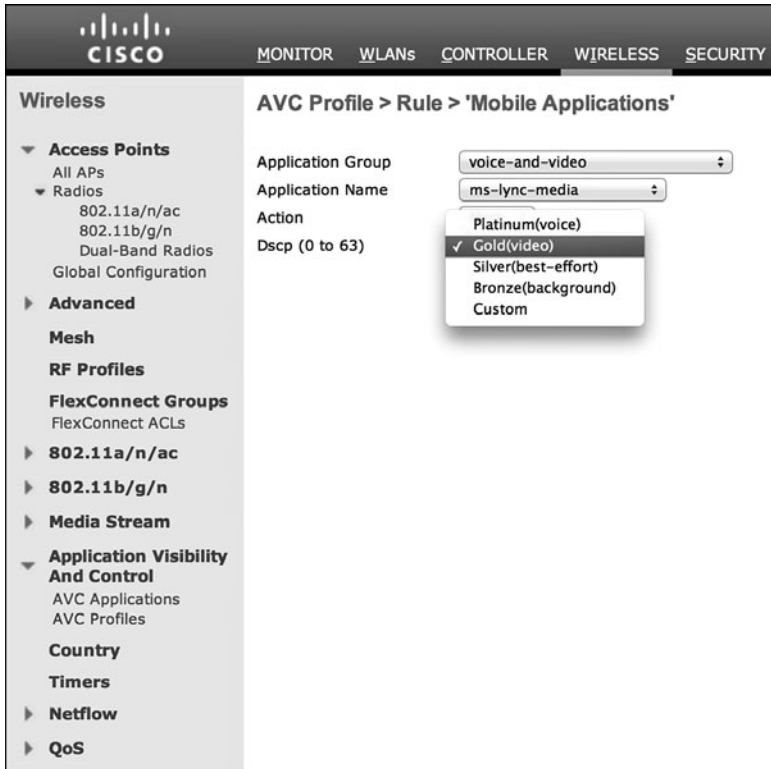
Figure 19-13 Re-marking DSCP Using AVC
