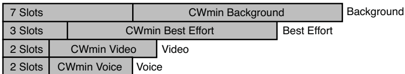
Figure 18-5 AIFS and Contention Window Sizing
