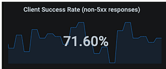
Figure 10.14 The client success rate shows that approximately 30% of requests are failing.
