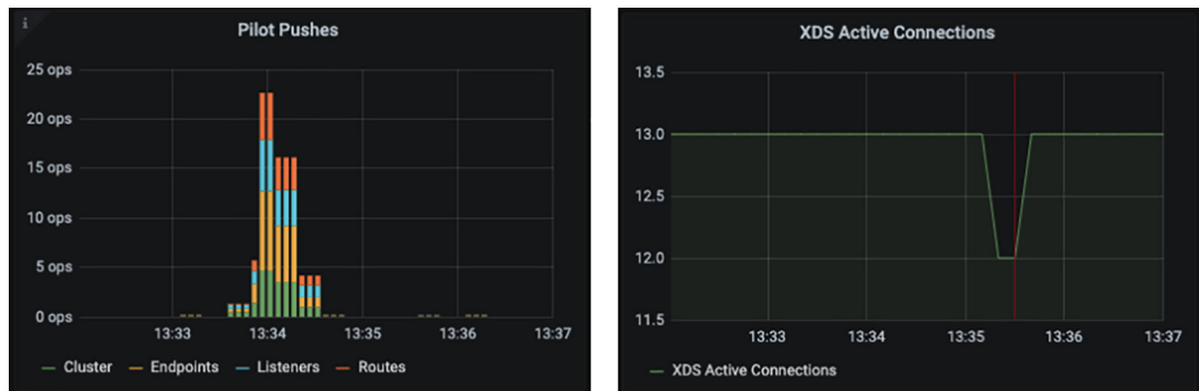
Figure 11.7 The Pilot Pushes graph shows the frequency of pushes. The XDS Active Connections graph shows the endpoints managed by a control plane.
