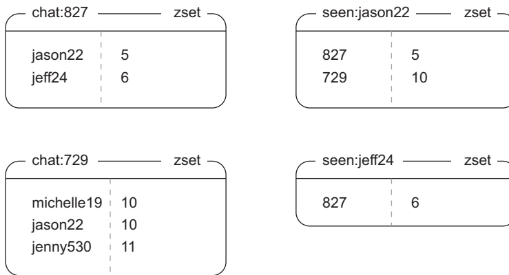
Figure 6.12 Some example chat and user data. The chat ZSETs show users and the maximum IDs of messages in that chat that they've seen. The seen ZSETs list chat IDs per user, again with the maximum message ID in the given chat that they've seen.
