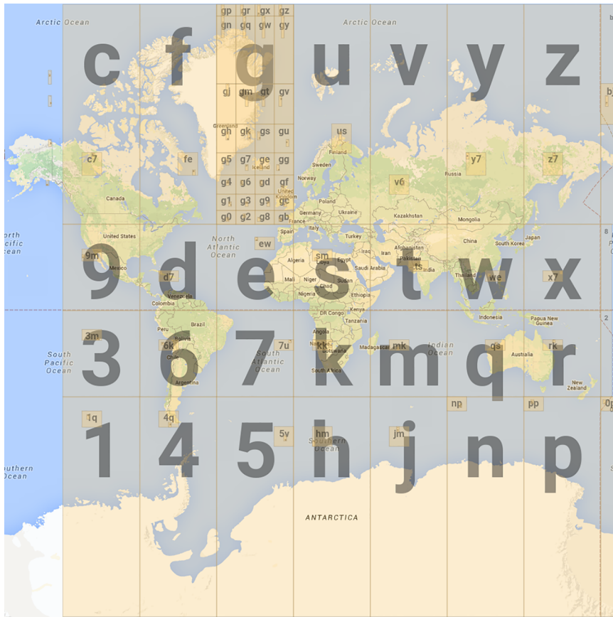
Figure A.3 The world divided in 32 letter-coded cells. Each cell is divided into 32 cells and so on, making longer hashes.
