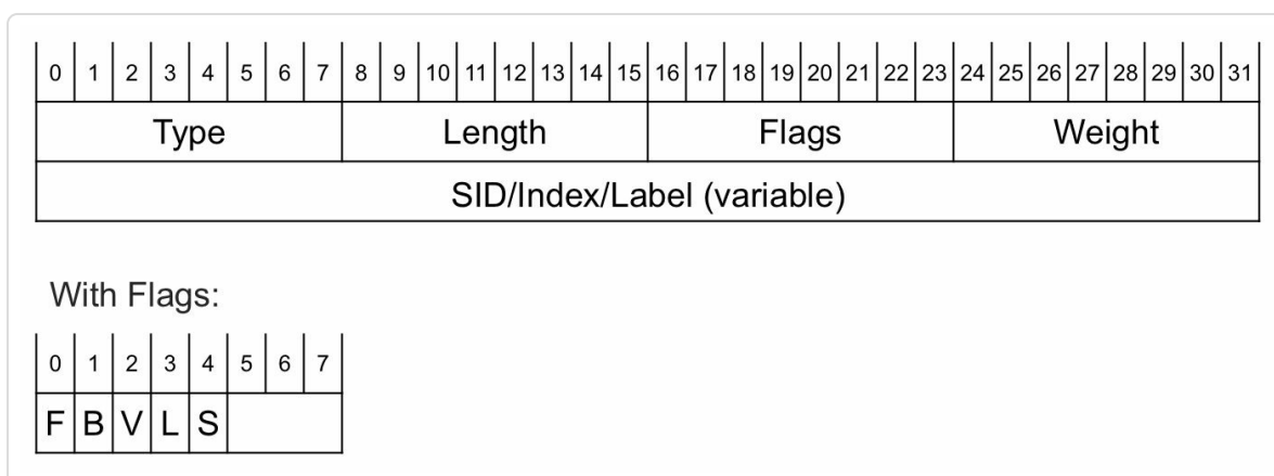
Figure 5-23: ISIS Adjacency-SID sub-TLV format
